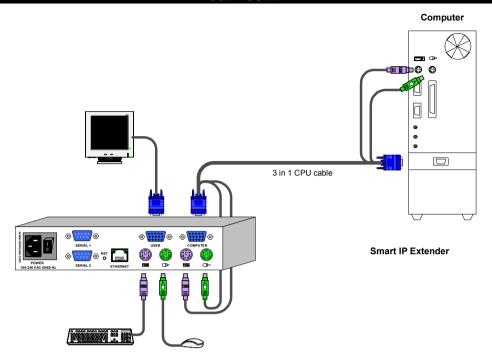
Figure 5 IP Extender connections to a computer
